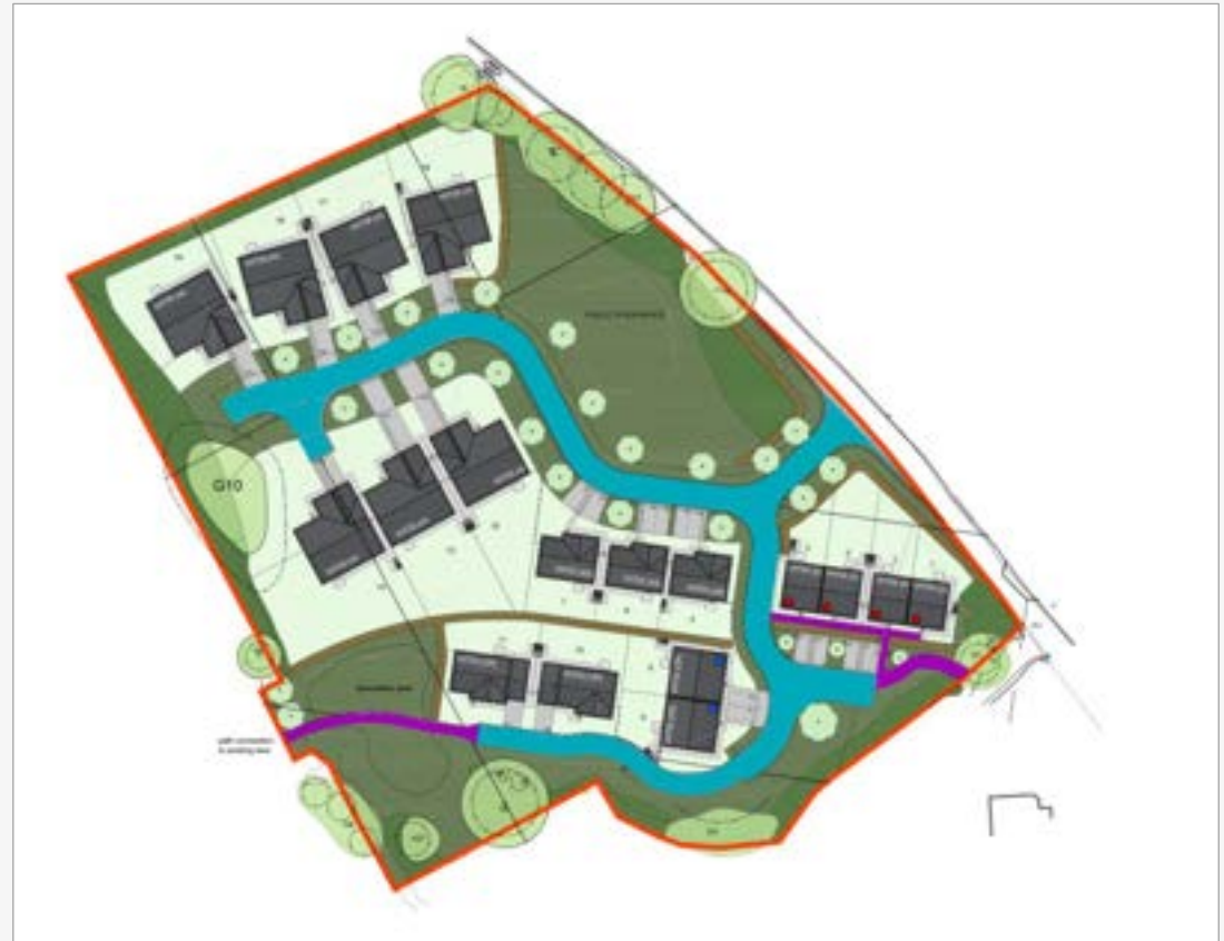
Fig. 13: Site plan showing vehicle and pedestrian routes. Blue – Roads Purple – Pedestrian routes
