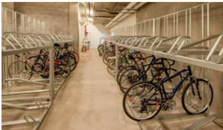
Example of internal bike = storage with double stacker's solution to double the amount of provided storage.
